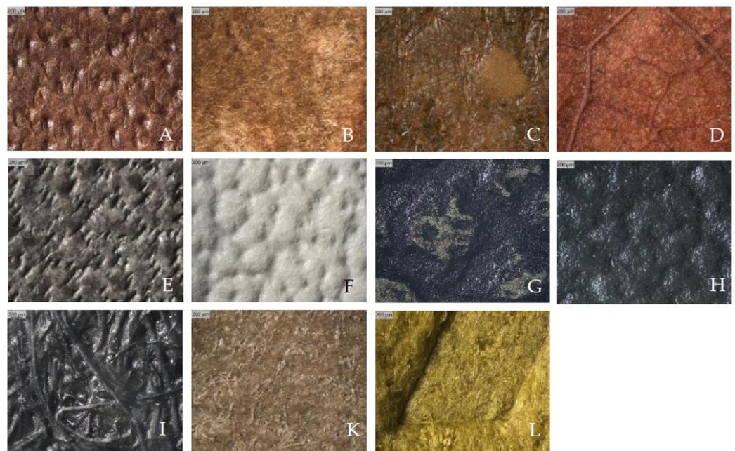
**Figure 3.** Surfaces of the investigated materials: Naturally grown material (Leather (A), Muskin<sup>®</sup> (B), Kombucha (C), Teak Leaf<sup>®</sup> (D)); embossed surfaces of coated textiles (PUR-coated textile (E), Desserto<sup>®</sup> (F), Appleskin<sup>®</sup> (G), Vegea<sup>®</sup> (H)); fiber structures of non-woven natural fibers (Pinatex<sup>®</sup> (I), SnapPap<sup>®</sup> (K)), and micro-fiber material (Noani<sup>®</sup> (L), embossed).
